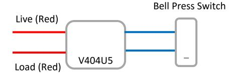
Connect the red wires to live and load respectively – the wires can be connected any way around.
