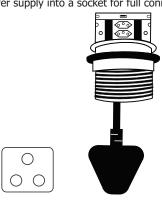
**Step 2**Unscrew and Remove Fixing Ring
