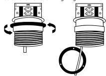
**Step 4**Replace fixing ring and tighten to ensure tight fit
